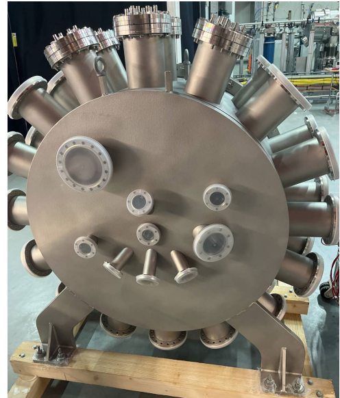
Figure 1: SpeAR vacuum chamber built by Just Vacuum and delivered to the European XFEL in Hamburg.
