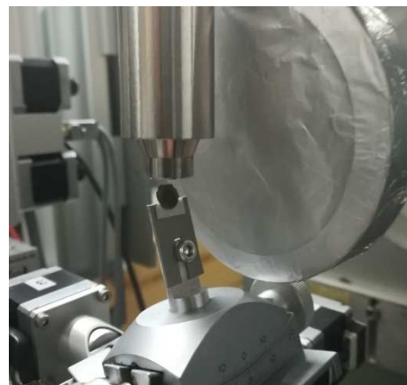
Fig. 1. Sample environment for XANES/EXAFS measurements, showing the cryo-nozzle (top), a mounted pellet and the TFY-diode (right).
