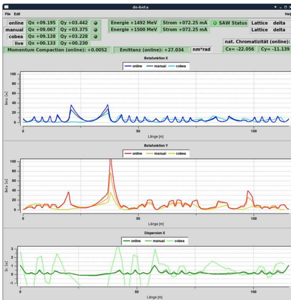
Fig. 1: Comparison of optical-function calculations based on online (i2k-converted) and manual values (e.g., design parameters) as well as COBEA results. In addition, the corresponding data of online mode simulations together with live tune measurements are displayed.
