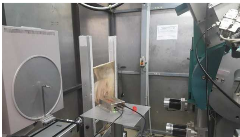
Fig. 1: Experimental setup for materials characterization at beamline BL9 of DELTA. The fluorescence detector analyzes X-ray fluorescence in backscattering and the MAR345 detector (left) acquires diffraction pattern in transmission geometry. The painting is mounted on horizontal and vertical translation stages.
