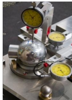
Figure 2: Dial indicators measuring the position of a Taylor Hobson placed on an alignment plate.
