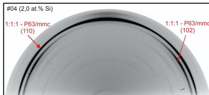
Figure 1: 2D diffraction pattern of the thin film measurement region with ~ 2at.% Si. The two most prominent diffraction signals are correlated to the CoMnGe HT phase.
