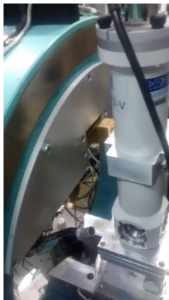
Figure 1: Left: The cryostat is mounted on a Huber Z-stage and connected to the diffractometer via ball bearings to minimize vibrations to the system. Right: Measured (004) Bragg rod of the 120 K sample. The relative changes between the Bragg peak position of the GaAs substrate and GaMnAs layer \Delta\theta are investigated.
