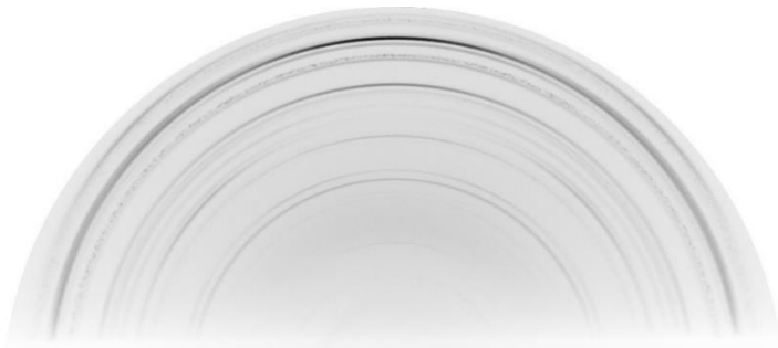
Figure 3: 2D synchrotron GI-XRD pattern for Fe-Si-Ge ternary with high proportion of Ge.
