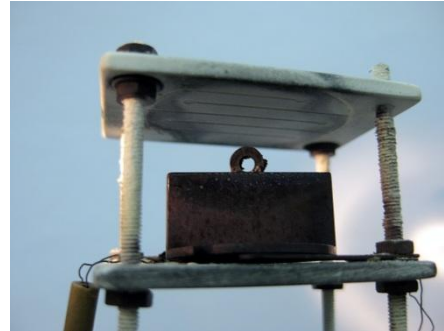
Figure 3: Heating elements and sample holder with sample [4]
