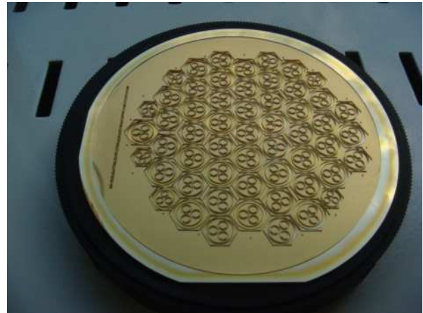
Figure 1: 4-inch Wafer with microgear structure after exposure, post exposure bake and development.
