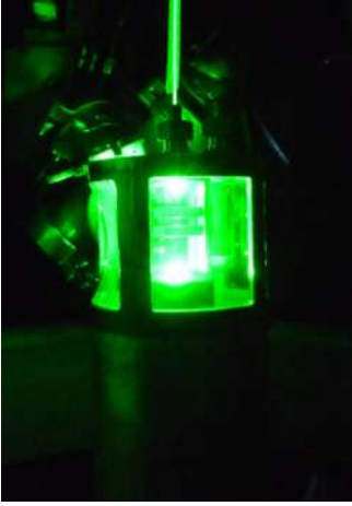
Figure 1: Picture of the in situ cryogenic sample cell. A lens system focused the Nd:YAG laser light on the sample.
