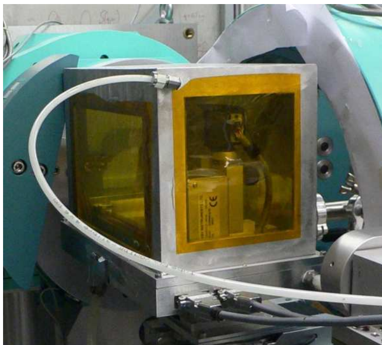
Fig. 2: The picture shows the sample cell, which was installed in the six circle diffractometer of BL9 in order to store the samples under a water saturated helium atmosphere.
