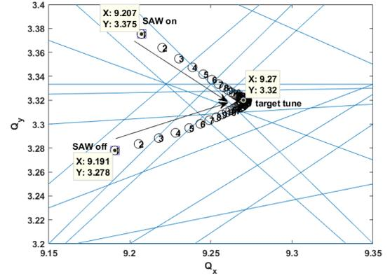
Figure 3: Two tune matching examples starting from different values with the wiggler magnet (SAW) switched on and off. The ML-based method calculates iterative shifts of the working point ( $Q_{x,y}$ ) up to an arbitrarily chosen target tune. The blue lines indicate resonance lines in the tune diagram up to the fifth order.
