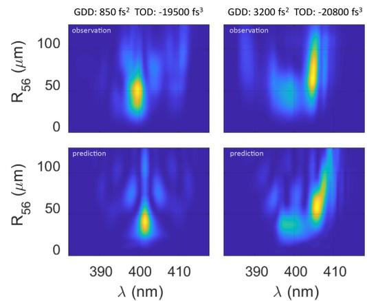
Figure 7: Observed CHG spectral maps (top row) and simulated spectral maps from the GDD and TOD values predicted by CNN (bottom row). The predicted GDD and TOD values are specified above each column.
