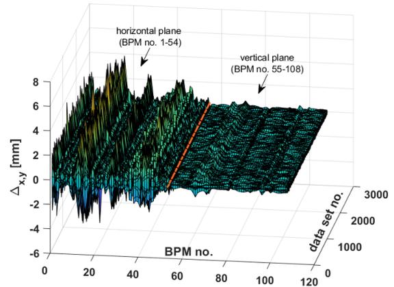
Figure 1: Orbit response at 108 BPM signals for the simulated  $x,y$ -coupled DELTA storage ring, calculated for 54 horizontal ( $x$ ) and 54 vertical ( $y$ ) deviations. In this example, 3000 randomly disturbed orbit vectors are shown. The data sets are used as inputs for supervised training of NNs.
