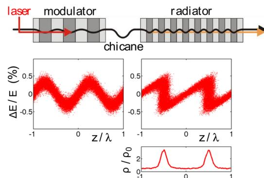
Figure 6: Magnetic setup for CHG, corresponding longitudinal phase space distributions and final longitudinal electron density.
